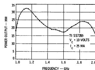
FIG. 4 - YIG Tuned Oscillator Power vs Frequency
