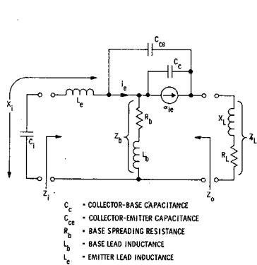
FIG. 1 - Transistor Oscillator Equivalent Circuit
