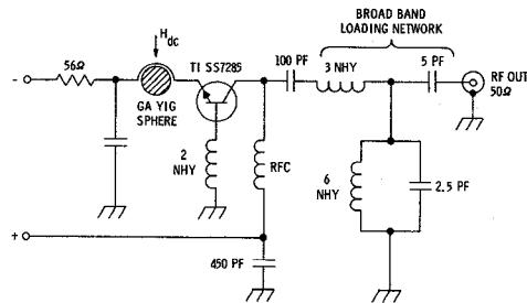
FIG. 3 - YIG Tuned Oscillator Circuit
