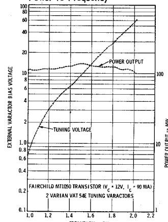
FIG. 6 - Varactor Tuned Oscillator Data
