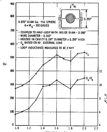
FIG. 2 - Measured YIG Resonator Q Data
