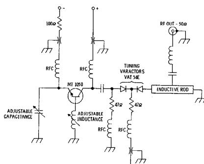
FIG. 5 - Varactor Tuned Oscillator Circuit
